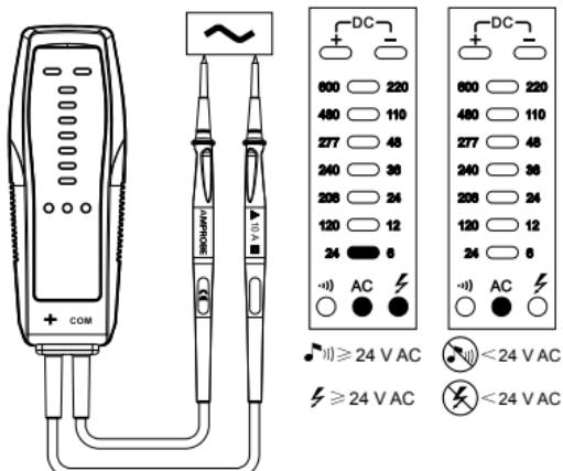
Figure 1: AC Voltage measurement
