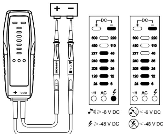
Figure 4: -DC voltage measurement
