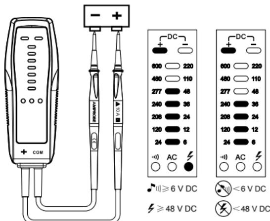
Figure 3: +DC voltage measurement
