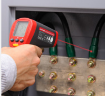
For precision measurements requiring the highest accuracy, emissivity can be adjusted for a wide range of material types (IR-720, IR-730 and IR-750).
