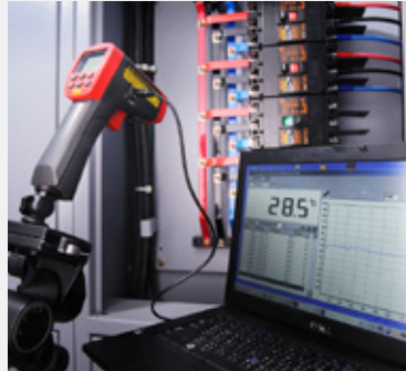
The advanced IR-750 records up to 99 data points for minimum, maximum, average, and hold, and has a USB port to export data for extensive analysis.
