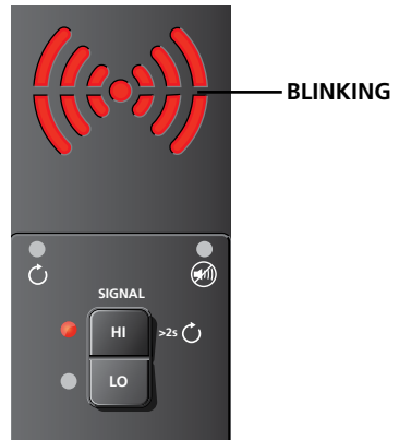
Figure 4.12b: Transmitter indicator showing signal in Loop mode
