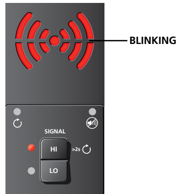
Figure 3.1b: Transmitter indicator showing signal in HIGH mode
