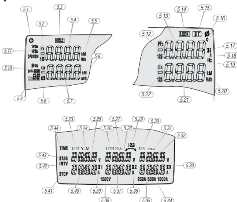
The multi-function display contains the currently measured primary quantities. The display format and the units (V, kV, A, kA, W, kW, MW etc...) are automatically displayed in compliance with the selected values.
