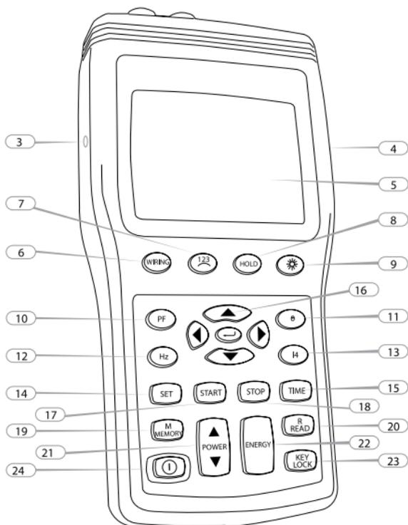
Figure: Front view – operation elements
