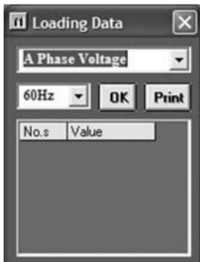
Select the requested input signal in the (A) window via the arrow keys.
