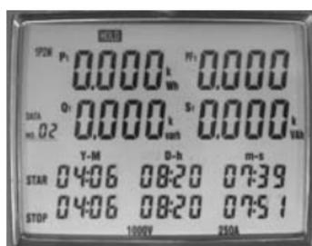
Display Measurement type energy in the lower part, the starting time of the measurement is displayed in the "STAR" line (5.43). Below, the current date and time are displayed during the measurement. I.e. the energy values are permanently calculated during running display. In the upper part of the display, the total values for the active power (5.4), the idle power (5.7), the apparent power (5.21), and the power factor (5.13) are displayed (to be recognised by the suffix "t") .
