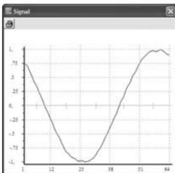
The values of the 64 sampling values are listed under No.s. In addition, a window with the representation of the signal curve will be displayed during the measured time interval of 20 ms (at 50 Hz).
