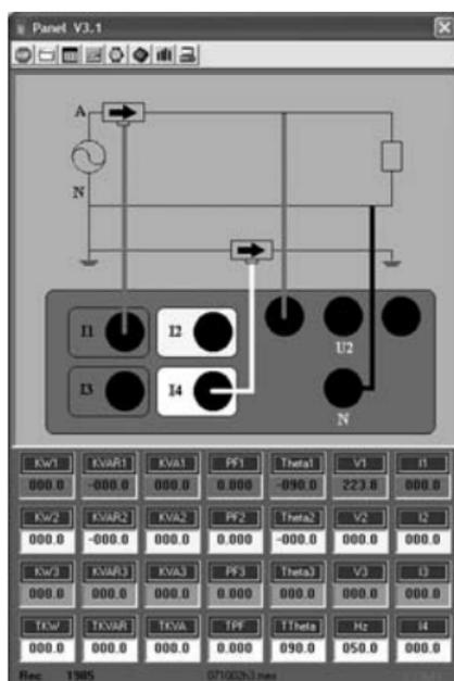
For checking purposes, the number of the already saved measured values and the file name are displayed in the line at the bottom.
