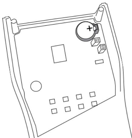
ⓘ The correct polarity of the batteries is indicated on the rear case. The connection "+" must be on the upper side.
