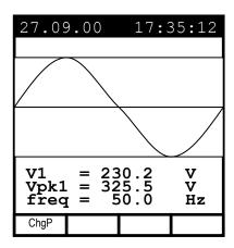
Example of screen in "4-wire" three-phase system
