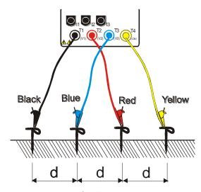
Instrument connection for Earth resistivity measurement
