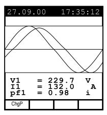
Example of screen in "4-wire" three-phase mode
