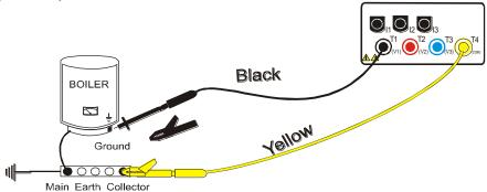
Connection of the test leads during LOW $\Omega$  test.
