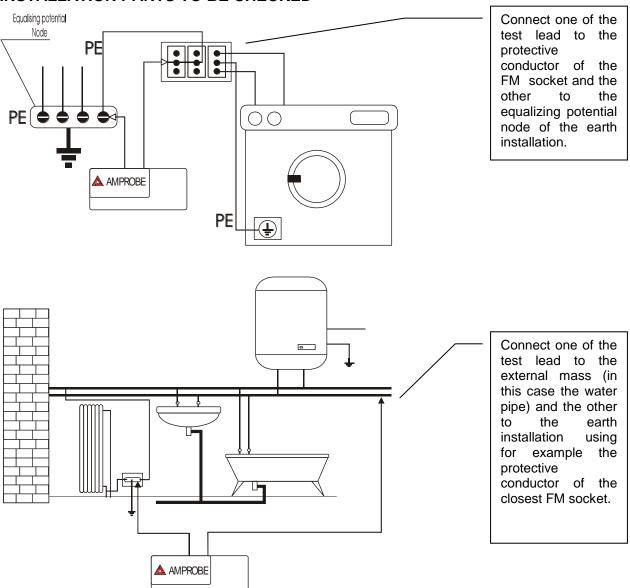
**Examples for continuity measurement on conductors**
