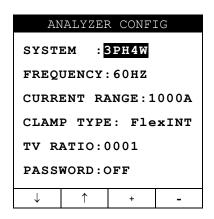
This page of setting can be confirmed by pressing the **ENTER** key or cancelled by pressing the **ESC** key.
