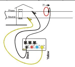
Instrument connection in a single-phase system
