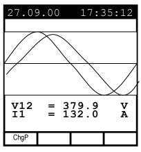
Example of screen in "3-wire" three-phase mode
