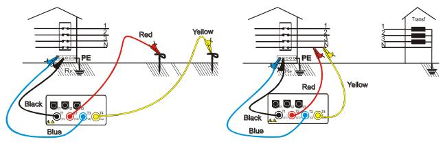
Connection for 3 point Earth resistance measurement
