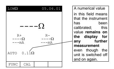
5. At the end of the test the result is stored and used as **OFFSET** (that is to say that it is subtracted from any continuity test carried out) for all the subsequent measurements.
