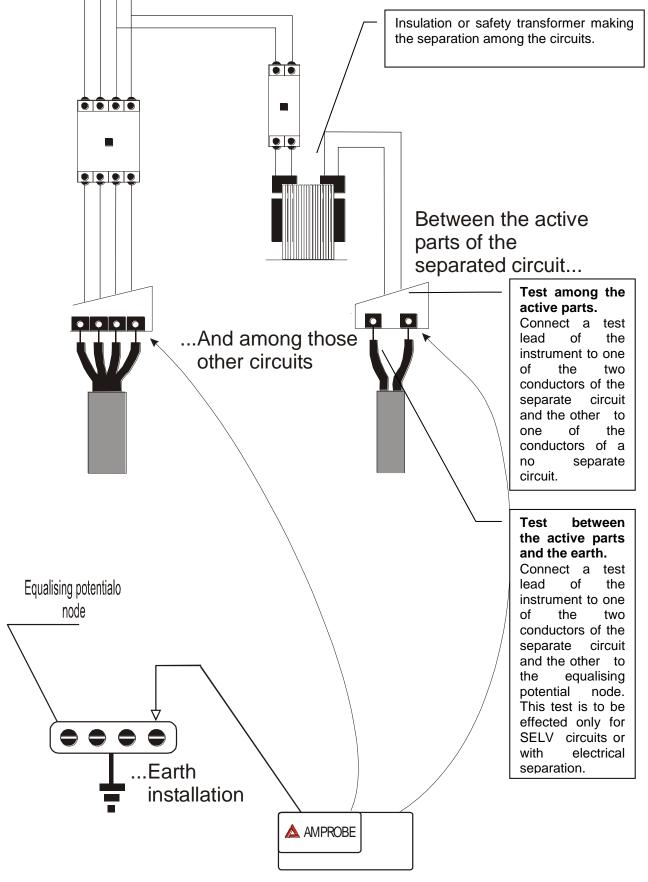
Measurement of separation among the installation circuits
