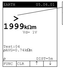
Message ">1999" means that the resistivity value is higher than the maximum measurable.
