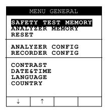
It's not possible to enter the **MENU** during a recording or a Real Time Energy measurement.
