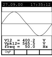
Example of screen in "3-wire" three-phase system
