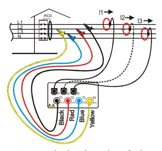
Instrument connection in a three-phase 3-wire system
