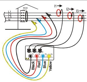
Instrument connection in a three phase 4-wire system
