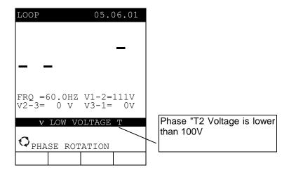
In the "Q" mode, if the instrument detects two phases connected together it displays the screen to the right.
