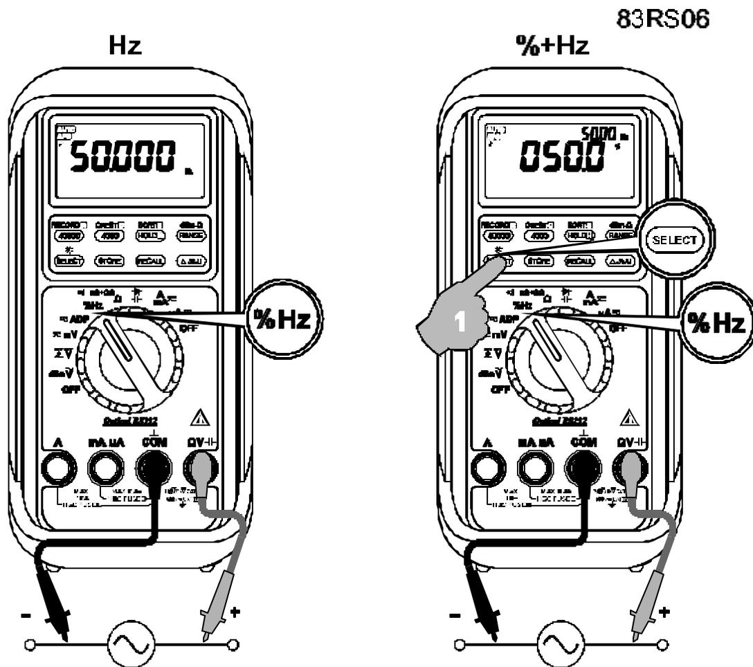
Note: Unlike the AC + Hz function, this high resolution Hz function is set at the highest input sensitivity to measure digital type electronic signals.
