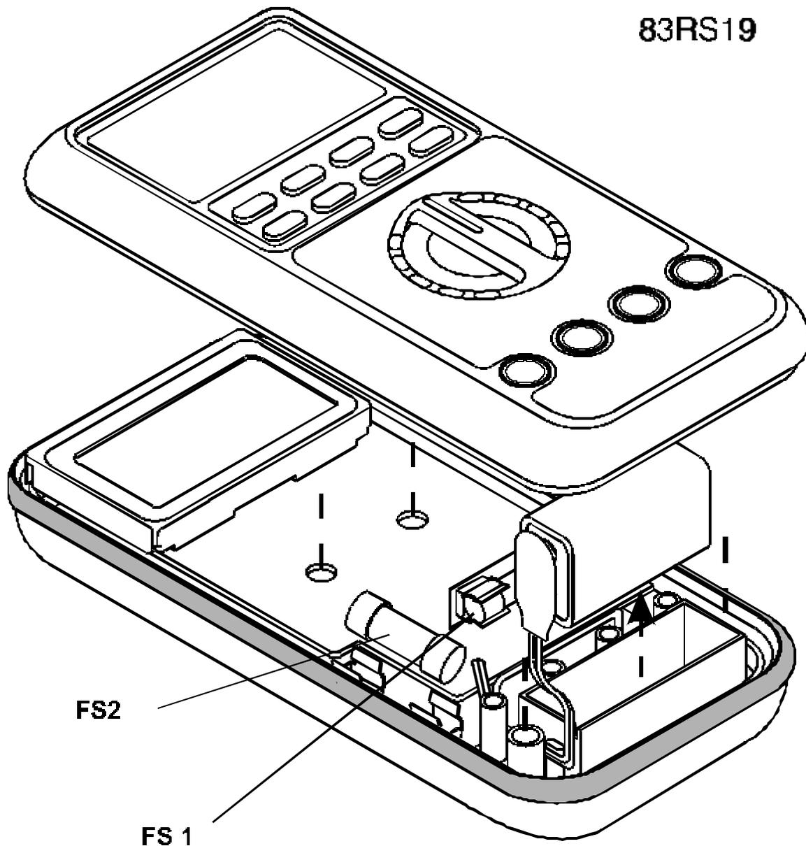
Loosen the screws from the case bottom. Lift the end of the case bottom nearest the input jacks until it unsnaps from the case top. Replace the battery and the blown fuse(s). Replace the case bottom, and ensure that all the gaskets are properly seated and the two snaps on the case top (near the LCD side) are engaged. Re-fasten the screws.
