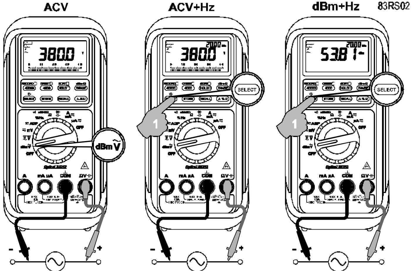
for measuring the frequency of high voltage noisy electrical signals.
