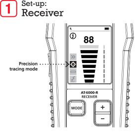
Turn on the Receiver. Press the MODE button to select a wire tracing mode (either Quick Scan or Precision Tracing). Tracing).
